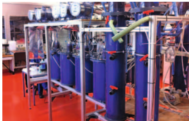
Figure 3: Status of trial on the anaerobic decomposition of pharmaceuticals from blackwater. Photo: Bauhaus University, Weimar
