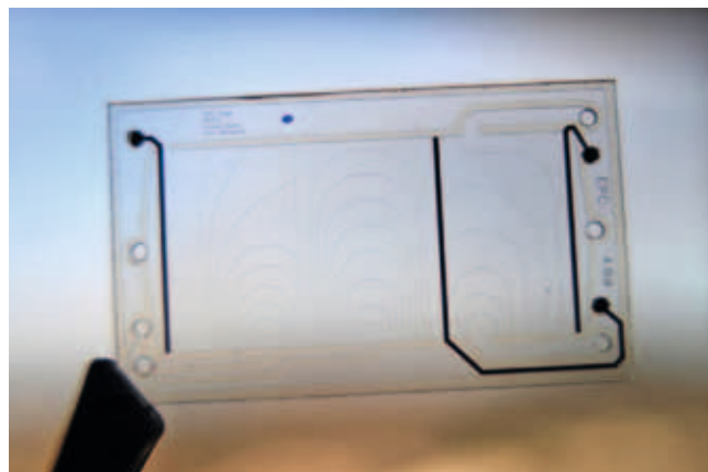
Figure 3: Implemented microchip in the lab-on-a-chip system. Photo: Gregory Dame
