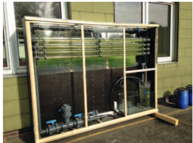
Figure 2: Piping system for algae cultivation – experimental plant. Photo: LimnoSun
