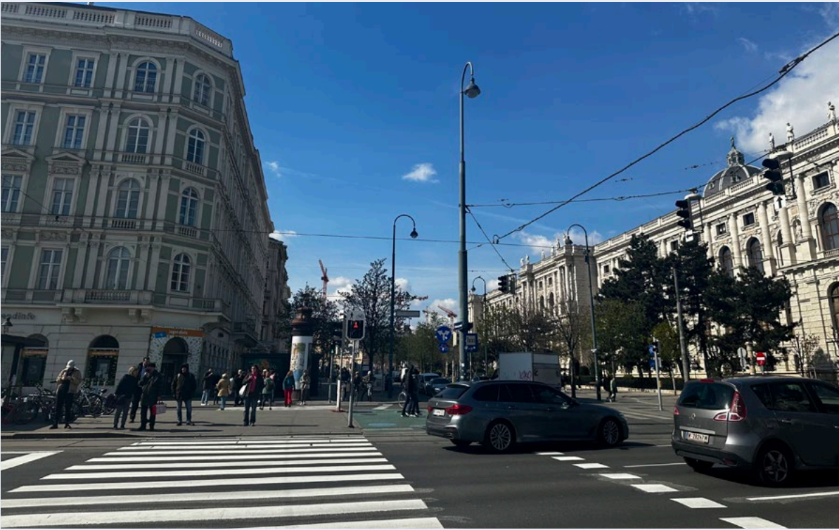
Figure 1: A pedestrian crossing in Vienna with a wide crossing and pedestrian refuge, clear pedestrian and bicycle signal, lighting, and a bicycle parking next to a covered bike shelter.
